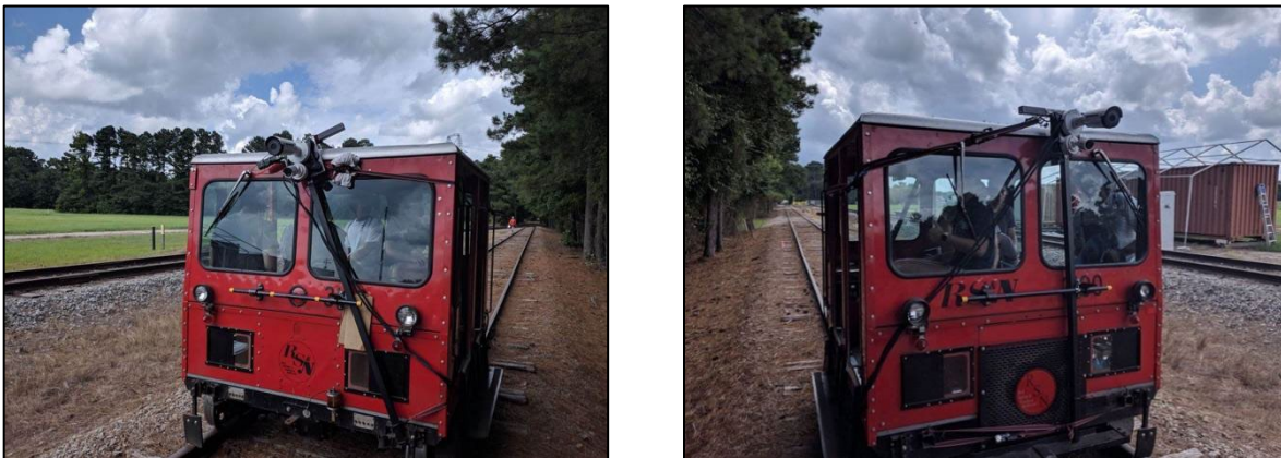
Figure 6. Camera Installation on Hi-Rail for Field Trial 2
