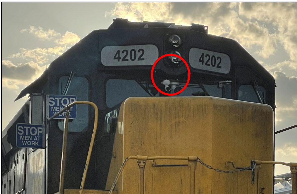
Figure 1. Example of Camera Systems Installed on a Train
