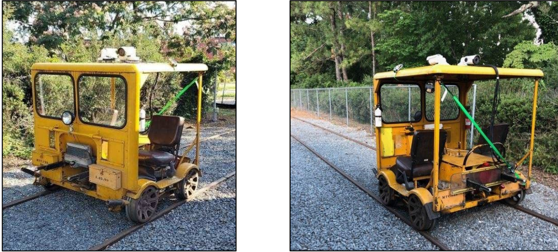
Figure 5. Camera Installation on Hi-Rail for Field Trial 1
